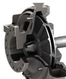
Semi-open and closed impeller design for slurry duty. Inducer for low NPSHa.
