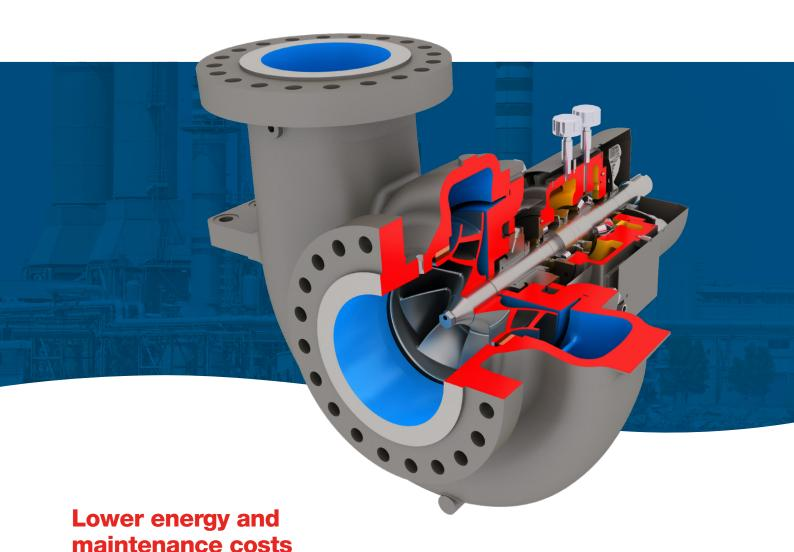
The Flowserve HHPX end-suction, single-stage, radially split pump is designed for high suction pressure seawater reverse osmosis (SWRO) desalination applications, such as energy recovery device (ERD) boosters. It is specifically engineered to deliver increased efficiency and easy maintenance, helping desalination plants lower energy and maintenance costs.
