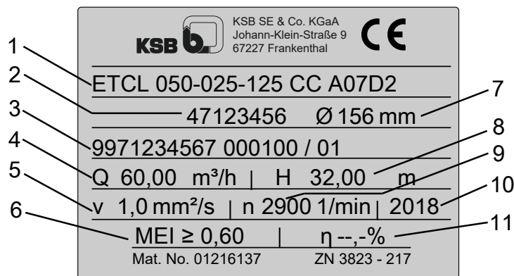
Fig. 5: Etachrom L name plate (example)
